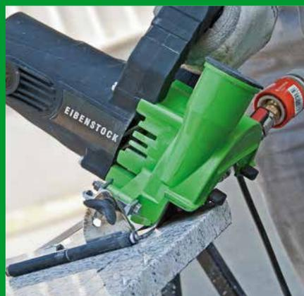
Cutting large-format slabs, mitre cuts up to 45°
