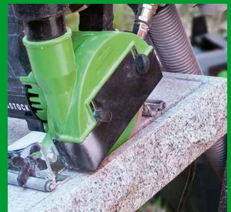
milling of joints with diamond milling disc – depth limiting and immersion function
