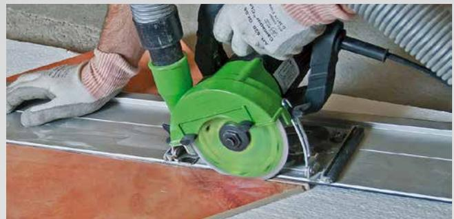
Machine on guide rail – for precise cuts, unlimited extensions
