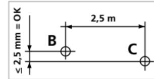
**!** Regularly check the calibration before use, after transport and after extended periods of storage.
