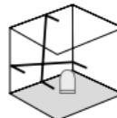
Do not release transport restraint, push slide switch (3) to the right. Sloping planes can now be measured. This mode cannot be used to perform horizontal or vertical levelling as the laser lines are no longer aligned automatically. LED (1) and the laser lines flash green.
