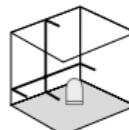
Release the transport restraint, push the slide switch (3) to the left. The laser lines can be switched individually with the selection button.
